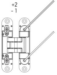
Within +2 mm (toward the hinges) / -1 mm. Horizontal adjustment is carried out on the part of the hinge installed in the door leaf. To make the adjustment, it is necessary to screw in or unscrew the two specified screws, using a 3 mm hex key, thereby setting the door leaf in the required position. It is not allowed to screw in or unscrew only one screw immediately to the extreme position, only sequential screwing.
