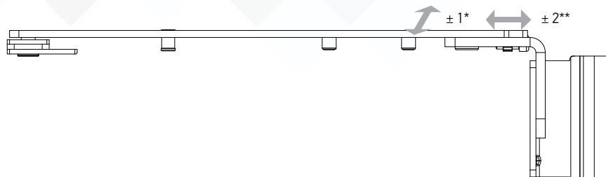
\* adjustment of gasket pressure, mm
